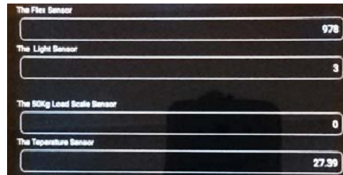
Fig. 17. The sensors values as they appear on the blind's Tablet when a true fall occurs.
